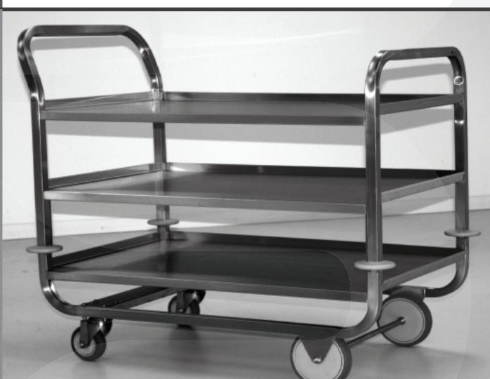
ERGONOMIC DESIGN HIGH LEVEL OF HYGIENE EASY TO CLEAN CONSTRUCTED OF STAINLESS STEEL 304, GRITT 320 ROBUST INTEGRAL FRAME CONSTRUCTION SHELF DIMENSIONS 860 X 530MM TROLLEY DIMENSIONS 1010 X 530 X 900MM 2 FIXED WHEELS 2 SWIVEL WHEELS FITTED WITH RUBBER BUMPERS FOR INTERIOR PROTECTION LOAD BEARING CAPACITY 30KGS PER SHELF
