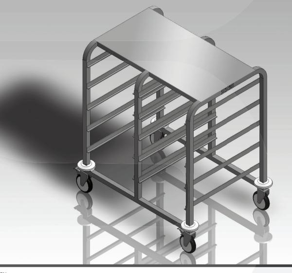
ERGONOMIC DESIGN HIGH LEVEL OF HYGIENE AND EASY TO CLEAN CONSTRUCTED OF STAINLESS STEEL 304, GRITT 320 ROBUST INTEGRAL FRAME CONSTRUCTION 2 FIXED WHEELS AND 2 SWIVEL WHEELS WHEEL BRAKES ANTI-DRUMMING PANEL FITTED UNDER THE SHELF RUBBER BUMPERS FOR INTERIOR PROTECTION SHELF DIMENSIONS 2 X 330 X 530MM CAPACITY 1/1 GN 530 X 325MM
