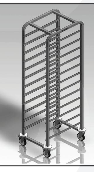
ERGONOMIC DESIGN HIGH LEVEL OF HYGIENE AND EASY TO CLEAN CONSTRUCTED OF STAINLESS STEEL 304, GRITT 320 ROBUST INTEGRAL FRAME CONSTRUCTION 2 FIXED WHEELS AND 2 SWIVEL WHEELS WHEEL BRAKES ANTI-DRUMMING PANEL FITTED UNDER THE SHELF RUBBER BUMPERS FOR INTERIOR PROTECTION SHELF DIMENSIONS 330 X 530MM CAPACITY 1/1 GN 530 X 325MM
