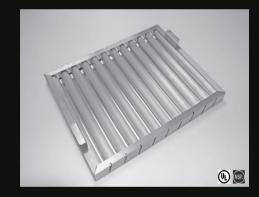
Vianen FECON® filters are constructed from stainless steel type 304 (DIN 1.4031 grit 320) 1.20 mm thick. The 36 mm thick filter is constructed without rivets and is provided with two integrated handles formed from the surrounding frame. On the top and bottom the filter 10% is open for the out stream of grease and moisture.
