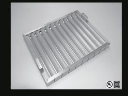
Vianen FECON® filters are constructed from stainless steel type 304 (DIN 1.4031 grit 320) 1.20 mm thick. The 36 mm thick filter is constructed without rivets and is provided with two integrated handles formed from the surrounding frame. On the top and bottom the filter 10% is open for the out stream of grease and moisture.
