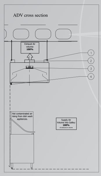
All metal edges are rolled smooth and are free from sharp edges and projections. The canopy lower edge is formed into a full perimeter condensation channel with inclined internal elevation to simplify cleaning and the inner edges are crush folded for safety purposes. Fitted directly under the duct spigot is a removable condensation plate. Drains in the gutter are optional. The canopy has a constant exhaust pressure drop of 40 Pa.
